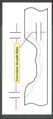
For reassessment, all the remaining strength methods are moot if future assumed corrosion rate wrong at site
